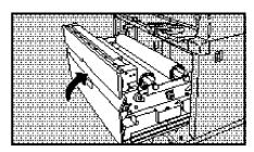
Turn the knob until the paper edge extrudes from the cover by about 150mm. 5.9" (cover closed).
